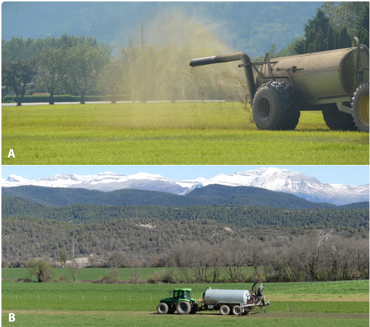
Image 16: Comparison of slurry spreading with a traditional 'splash plate' spreader ( A ), maximizing ammonia emissions, (photograph: © Shabtai Bittman) with a trailing hose manure spreader ( B , Field Measure 6) for reducing ammonia emissions, here deployed on-farm in a sensitive mountain landscape. For optimal performance, hose exits should be as low as possible within the canopy, though they may be raised when turning or transporting manure from the farm (photograph: © L'Albeitar, 2021).
