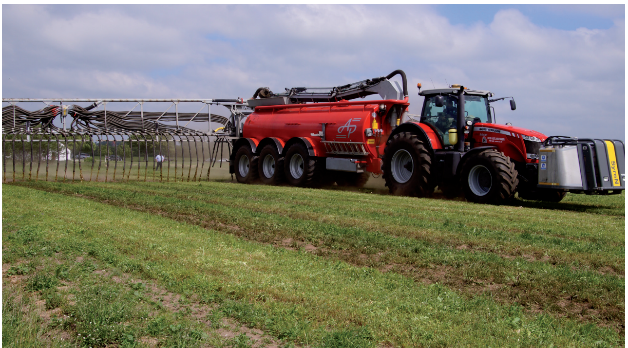
Image 19: In-field slurry acidification (Field Measure 9) lowers slurry pH to <6 reducing ammonia emissions. Sulphuric acid from the tank at the front of the tractor is added to the slurry at a controlled rate to achieve the desired pH during the spreading operation. North Jutland, 2013 (photograph: © BioCover).
