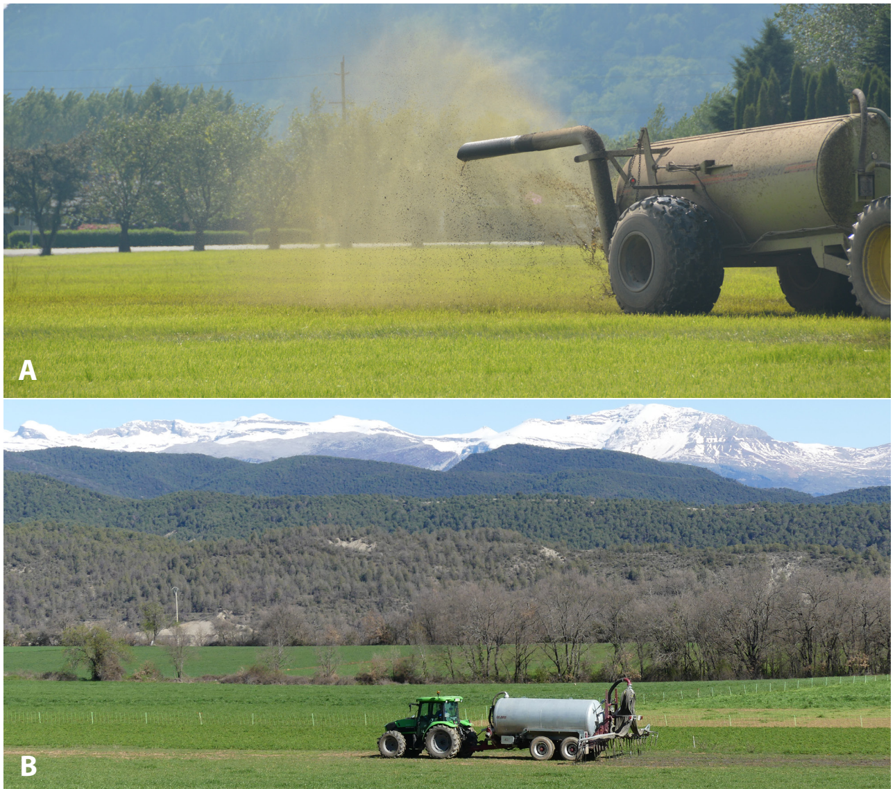
Image 16: Comparison of slurry spreading with a traditional 'splash plate' spreader ( A ), maximizing ammonia emissions, (photograph: © Shabtai Bittman) with a trailing hose manure spreader ( B , Field Measure 6) for reducing ammonia emissions, here deployed on-farm in a sensitive mountain landscape. For optimal performance, hose exits should be as low as possible within the canopy, though they may be raised when turning or transporting manure from the farm (photograph: © L'Albeitar, 2021).
