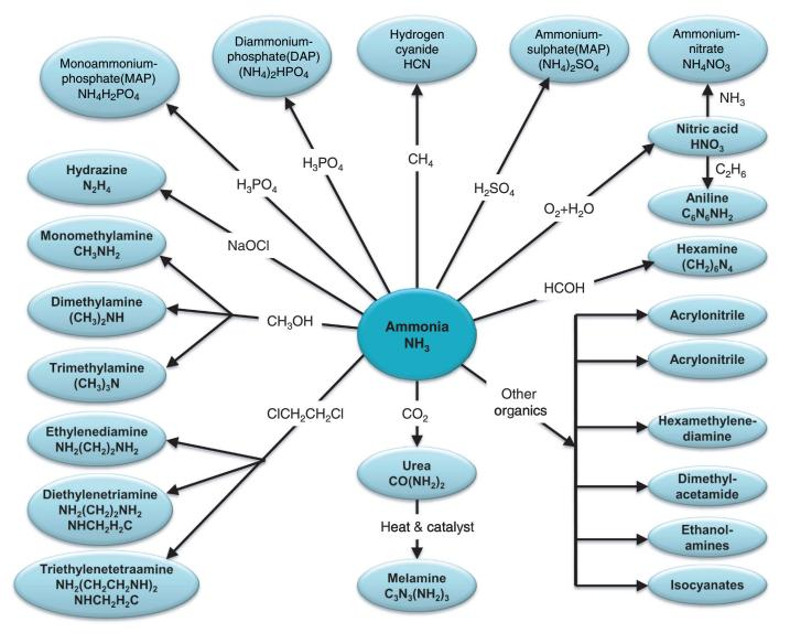
Fig. 3.19 Synthetic nitrogen products made from ammonia (modified from Maxwell, 2004).
